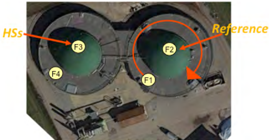
Fig. 2 The two investigated gasometric coverage systems at the biogas plant of the Cooperativa Speranza (Candiolo, TO)
