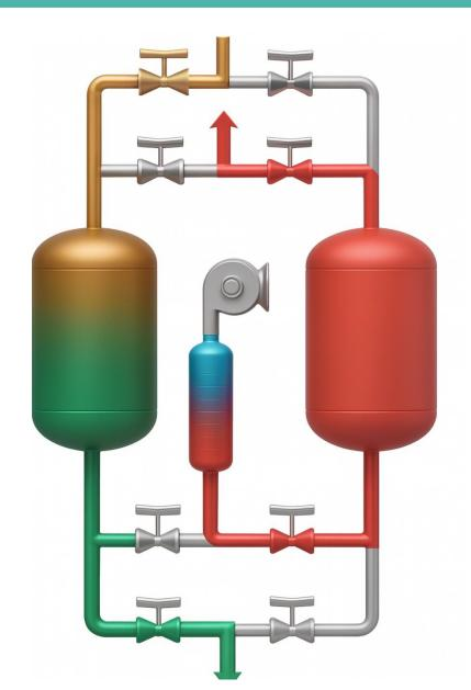
The untreated biogas which contains VOC & Siloxanes passes through the filter system and is fed to the gas engines up to 99% purified from VOC & Siloxanes.
